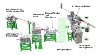
Fig.10 Schematic diagram of the IR beamline with the shield walls and experimental hutch removed
