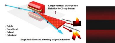
**Fig. 11**. Left: Schematic diagram illustrating the formation of bending magnet radiation. **Right**: The image of the radiations at the first mirror.
