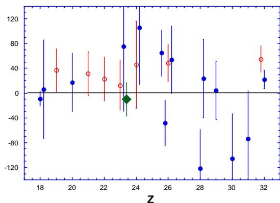
Fig. 1. Helium-like QED theory for the dominant  $w$  line ( $1s-2p$   $^1P_1-1s^2$ ) (Drake, 1988), atomic number  $Z = 15-40$  (straight line) versus PLT tokamak measurements and EBIT measurements by Beiersdorfer et al. (1989, open circles) compared to other experimental results (filled circles). Solid diamond is Chantler et al. (2000) where other references are also provided.
