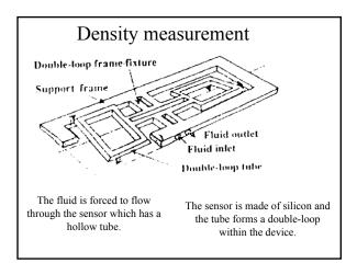
The tube inlet and outlet are at the side and the entire loop is designed for torsional vibration.
