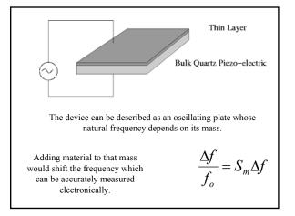
$\label{eq:F_0} F_{0} \mbox{=} the unloaded natural frequency, $\Delta f$ is the frequency shift, $\Delta m$ is the added mass per unit area and $S_m$ is the sensitivity factor.$
