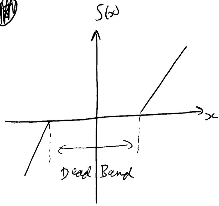
Dead band is the insensitivity of the sensor to a range of input signals
