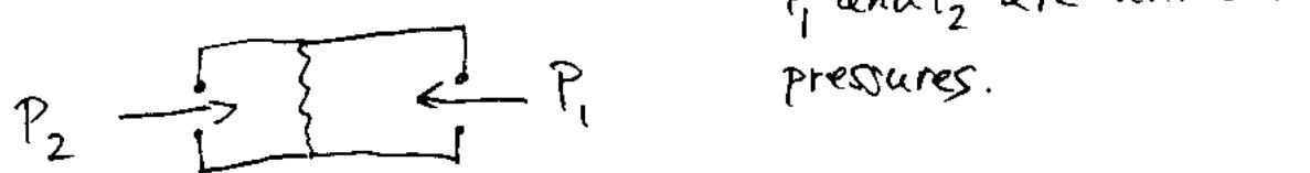
In all three cases, we measure the displacement of the membrane; by electrical or optical means, usually.
