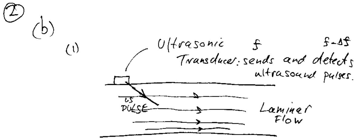
note that with Laminar flow the velocity is greatest at the middle and zero at the walls. We will get a range of Doppler shifts - we are interested in the maximum i.e.  $\Delta f_{\max}$ .
