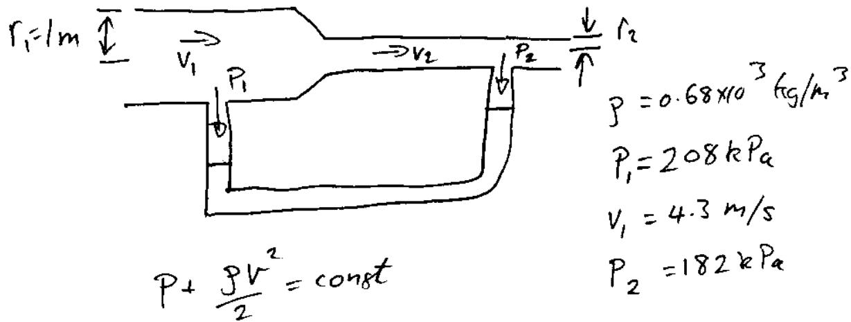
$$(a) \quad P_1 + \frac{1}{2} \rho V_1^2 = P_2 + \frac{1}{2} \rho V_2^2$$
