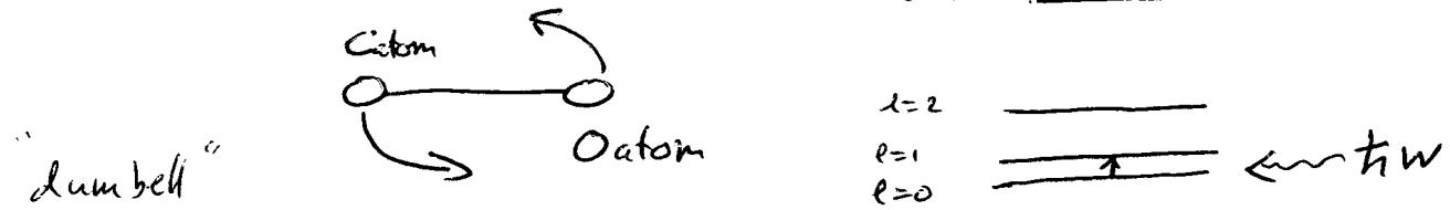
$\ell=0 \rightarrow \ell=1$  is an increase in energy of the  $\text{CO}$  molecule, so the energy that is added to the system must have come from an incident photon of energy  $\hbar\omega$ . (Note  $\hbar\omega = \frac{\hbar \cdot 2\pi f}{2\pi} = \hbar f$ ). The  $\ell=0$  rotational state has no energy  $E_{\ell=0}=0$ , i.e. the dumbbell is not spinning. After it has absorbed the photon, it is <sup>now</sup> spinning.
