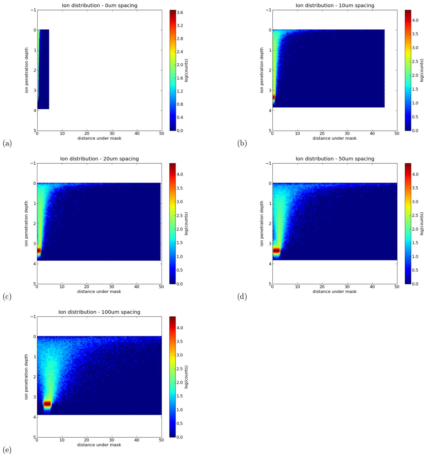
Figure 5: Ion distributions for various mask-target spacings with a narrow beam. Here a sharp beam was used to give more scattering from the mask, with the side effect that not many ions are recorded further out from underneath the mask (as the beam did not cover that area). ( $\sim 500\,000$  ions are visible in these plots)
