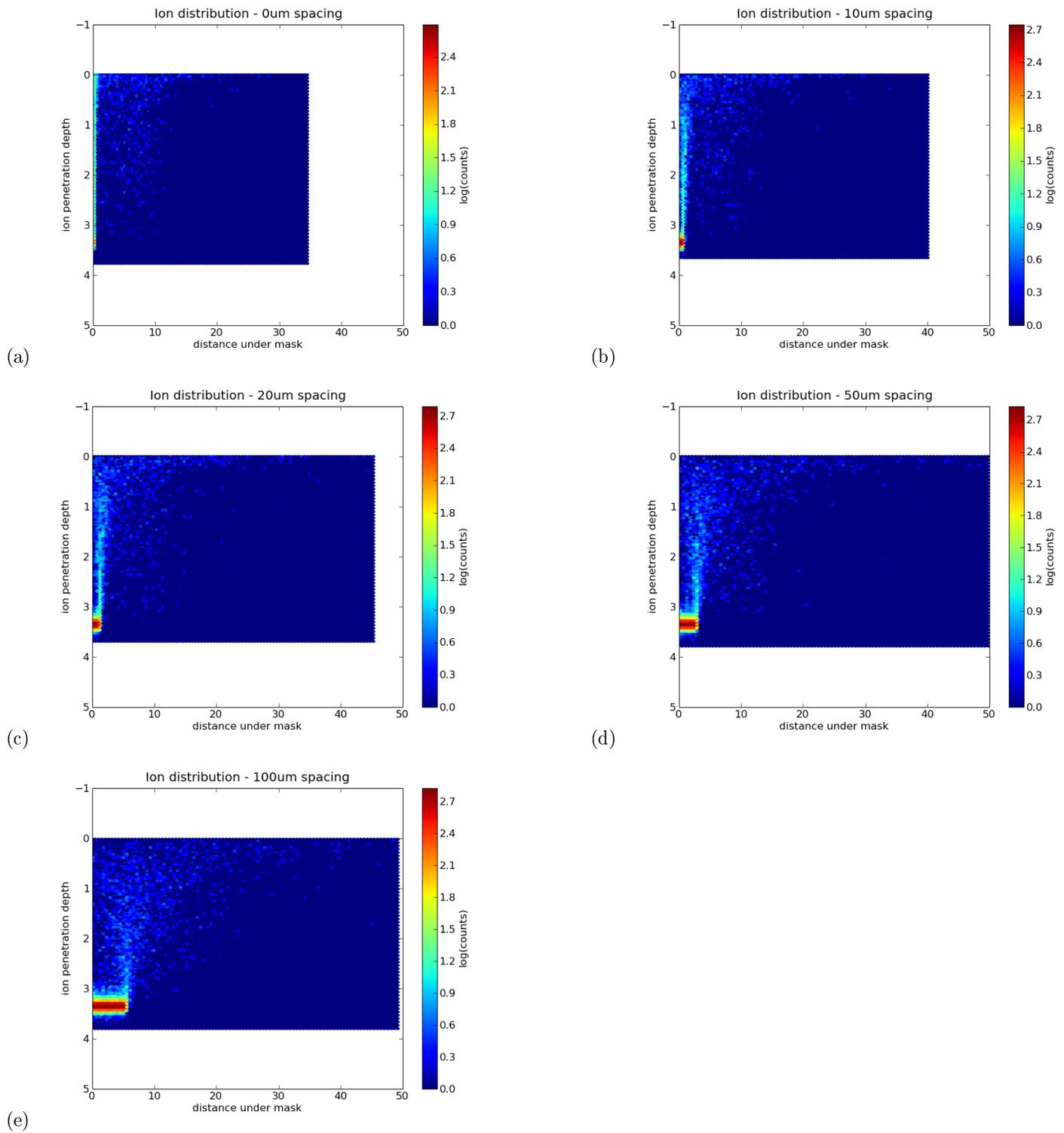
Figure 4: Ion distributions for various separations with a wide beam. A wide beam was used here so not many ions impacted the mask. ( $\sim 50\,000$  ions are visible in these plots)
