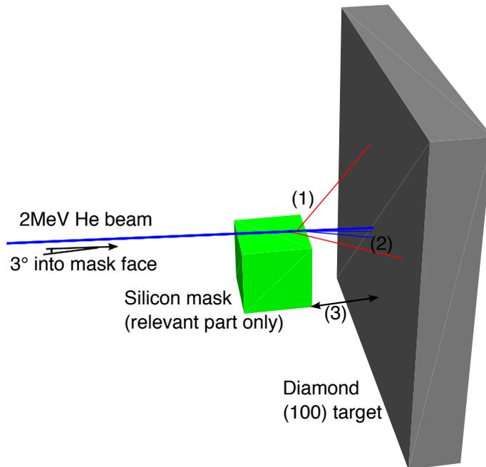
Figure 1: Diagram of experimental setup. The 2MeV He beam (blue) is directed at a 3° into the edge of a cleaved silicon mask. (1) He ions clip the edge of the silicon mask and are absorbed or scattered, also producing secondary electrons (red). Ions that don't hit the mask are not simulated. (2) Scattered ions hit the diamond target and come to rest. (3) The mask-target spacing is varied during the simulation (by moving the target).
