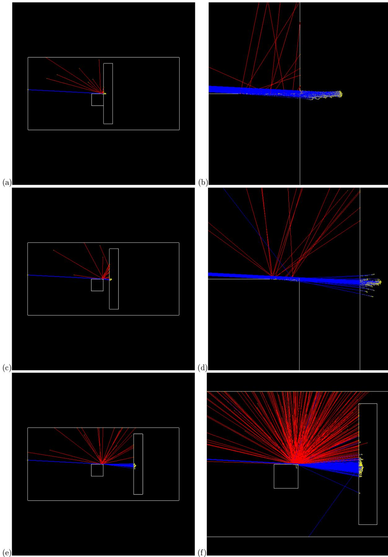
Figure 2: Various screenshots of simulations. Blue lines are ion tracks; red scattered electrons; yellow dots are energy deposits. (a) 0um gap. (b) Closeup of 0um gap impact site. (c-d) 10um gap. (e) 50um gap. (f) 50um gap closeup, with 1000 ions to show a high angle scattered ion (and also a reflected ion).
