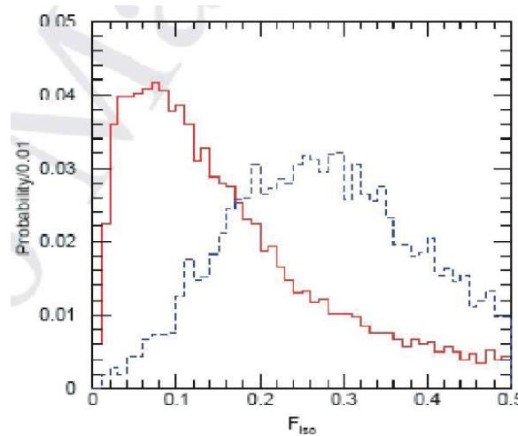
$$fracE_T^{R_{12}} = \frac{\sum E_T^{cell}(R_{1P,cell} < 0.2) - \sum E_T^{cell}(R_{1P,cell} < 0.1)}{\sum E_T^{cell}(R_{1P,cell} < 0.2)}$$
