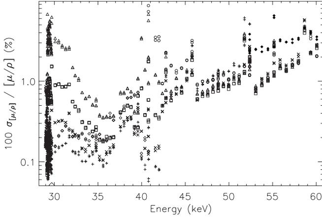
FIG. 4. Precision of the attenuation measurements as dominated by counting statistics recorded by the first downstream ion chamber. The uncertainty of  $\left[\frac{\mu}{\rho}\right]$  for the optimum foil thickness is of order 0.2% for measurements below 35 keV. Above this energy the declining x-ray flux and detector efficiencies leads to higher uncertainty levels. Symbols as for Fig. 3.
