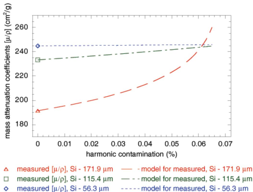
FIG. 2: Effect of third-order harmonic contamination in attenuation measurements using Si(111) monochromator and three silicon sample thicknesses at 5 keV. All three measurements are consistent with a unique percentage of third-order harmonic contamination of about 0.06%.
