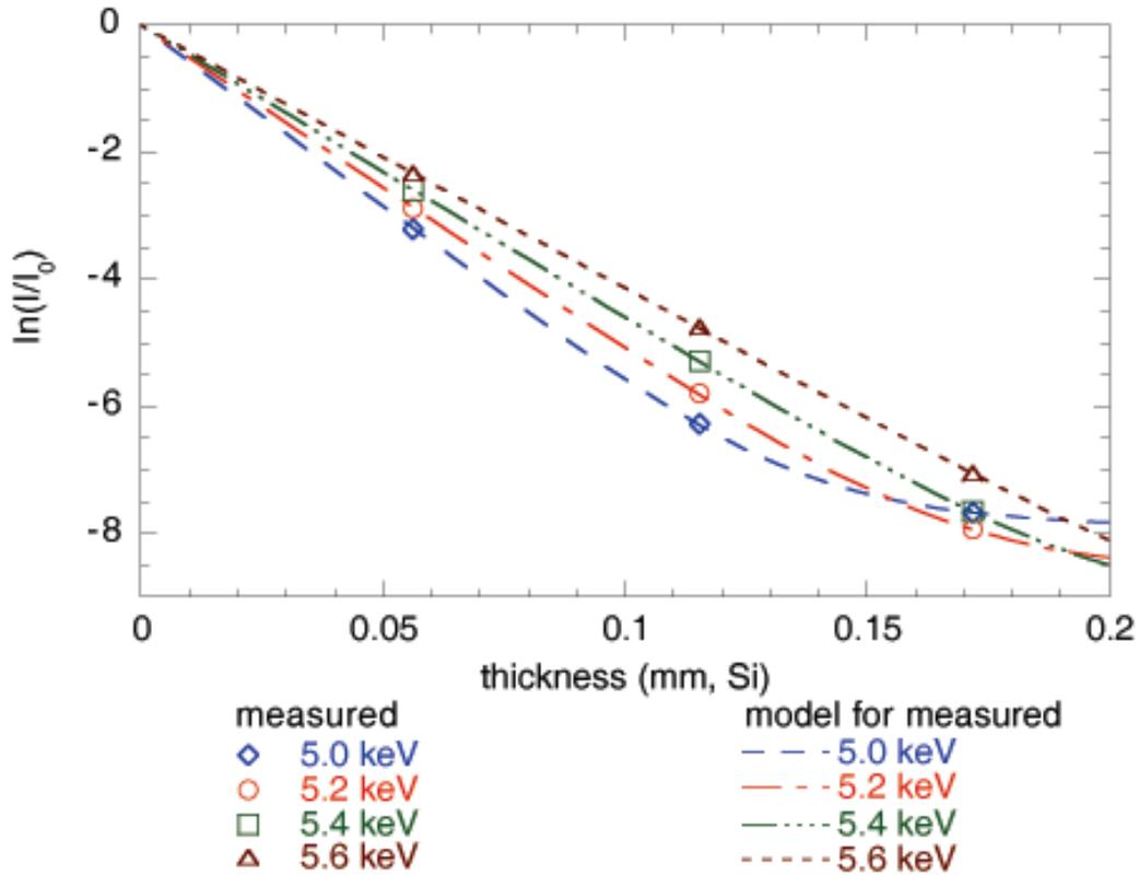
FIG. 3: A harmonic component measurement with three well calibrated thicknesses provides a constant and reliable indicator of accuracy in attenuation measurements. Error bars are given by the thickness of the line.
