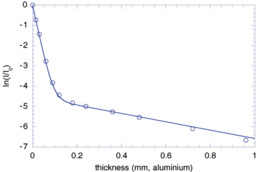
FIG. 1: The attenuation,  $\ln(I/I_0)$ , as a function of the thickness of aluminium absorber in the x-ray beam with a silicon monochromator set to 5 keV.  $\circ$  - experimental results; solid line - curve of best fit corresponding to an admixture of  $(1.09 \pm 0.02)\%$  third-order harmonic (15 keV).
