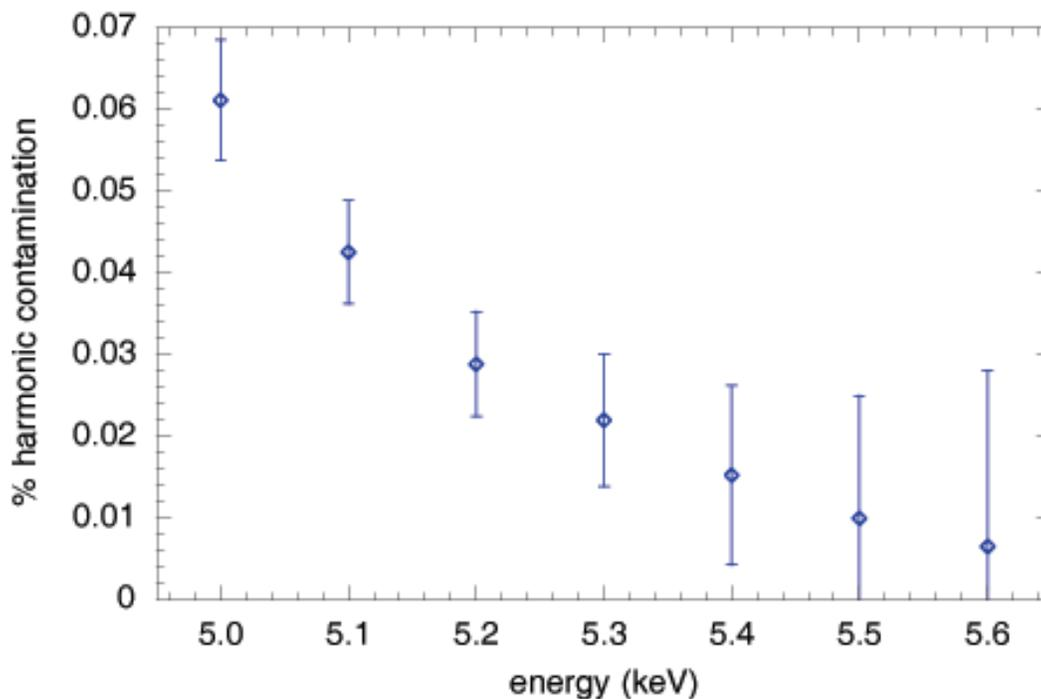
FIG. 4: Energy variation of the fraction of harmonic contamination in the example chosen (at maximum detuning).
